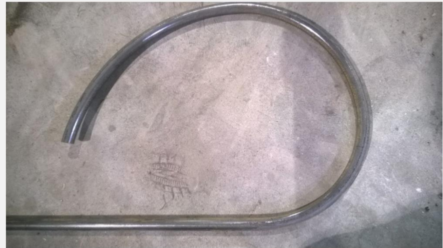
Hardox Tube 500 30 x 3 mm with radius 270 mm
